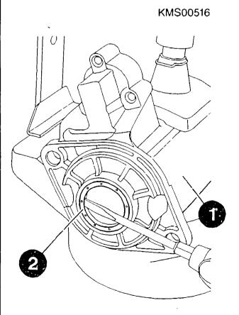
Checking drive-end bearing
